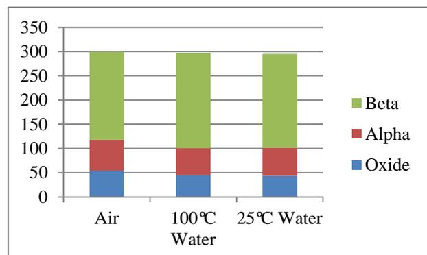
Fig. 5. Thicknesses of each phase layer. Air-cooled specimen had thickest oxide and alpha layer.
