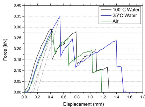
Fig. 6. Displacement-Force graph of ring compression test (RCT) in room temperature (20°C). Each claddings had 1.5%, 2.0%, 1.1% offset strain.
