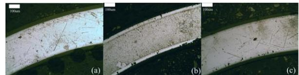
Fig. 4. Optical microscopy snapshot of phase layer in (a) air-cooled sample, (b)  $100^\circ\text{C}$  water-quenched sample, (c)  $25^\circ\text{C}$  water-quenched sample
