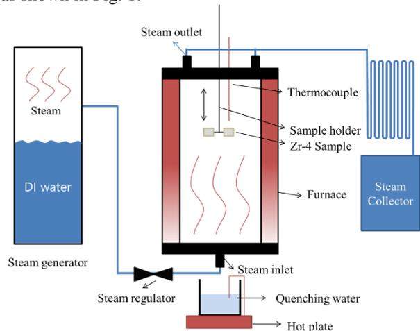
Fig. 1. Schematic of LOCA experimental set up
