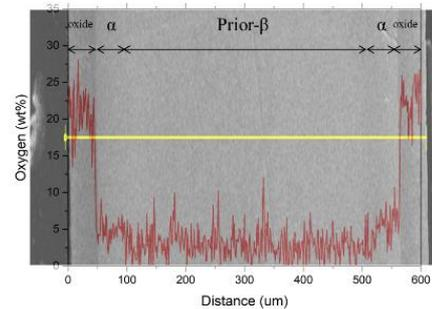
Fig. 3. Energy Dispersive Spectrometry (EDS) of phase layer. Oxide,  $\alpha$ , and prior- $\beta$  layer are shown.
