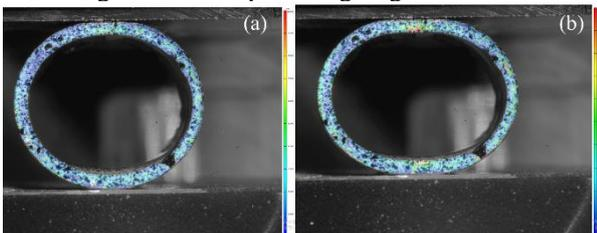
Fig. 7. Digital image correlation(DIC) analysis of cladding sample. (a) before failure (crack opening), (b) after failure of the sample.
