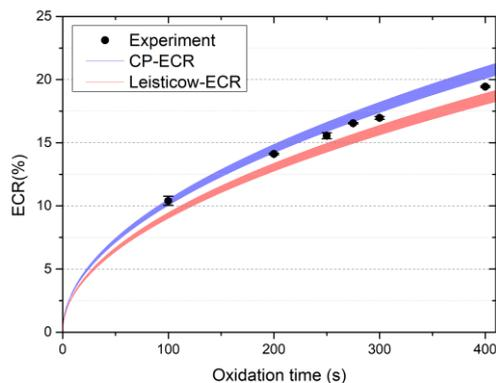
Fig. 2. Comparison between CP-ECR ( $1204 \pm 5^\circ\text{C}$ ) and mass-calculated ECR in this experiment
