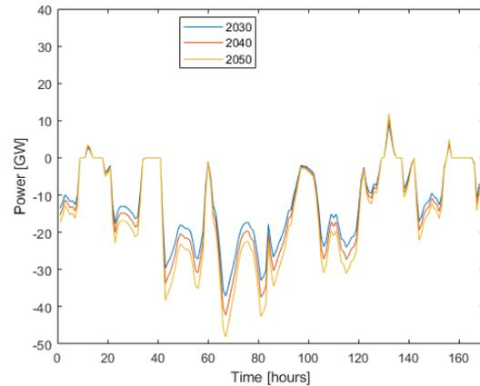
Fig. 4. Oversupply and undersupply of year 2030, 2040, and 2050 mitigated with ESS
