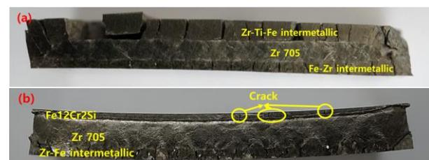
Fig. 5. Overall shape and each layer's chemical composition of small plate specimens after cold rolling: (a) 3-layer, (b) 4-layer
