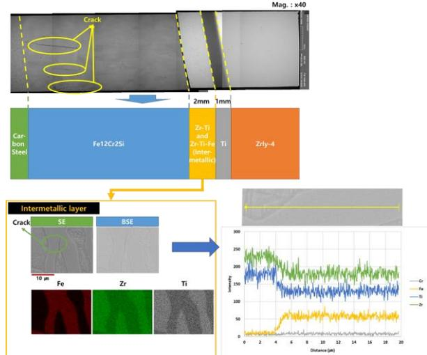
Fig. 7. EDS mapping and line-scan results on the cross-sectional images of 3-layer mother tube after HIP process
