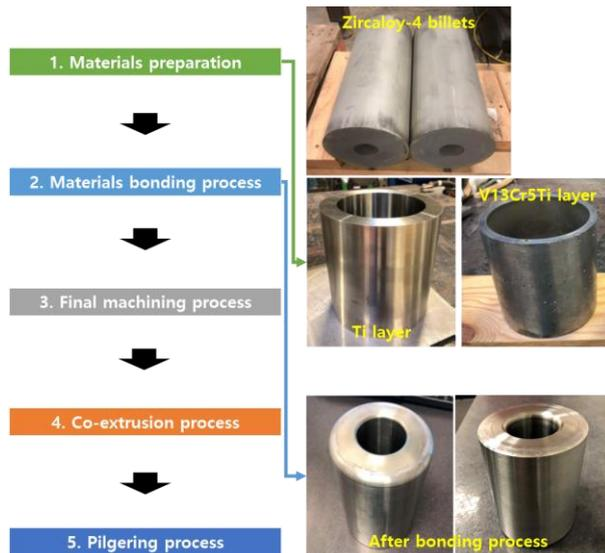
Fig. 8. Fabrication process and photographs of 4-layer mother tube
