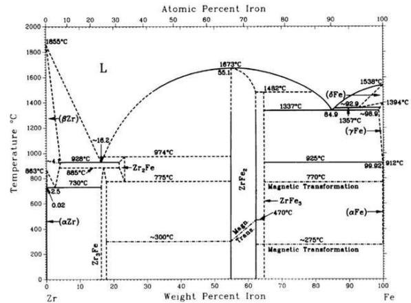
Fig. 1. Zr-Fe phase diagram [4]
