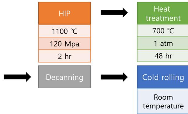
Fig. 4. Total process of small plate specimens
