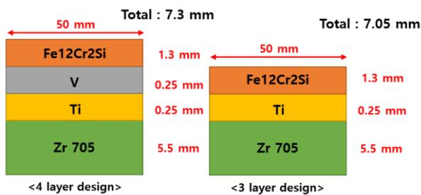
Fig. 3. Schematic of small plate specimens
