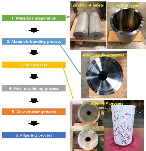
Fig. 6. Fabrication process and picture of 3-layer mother tube
