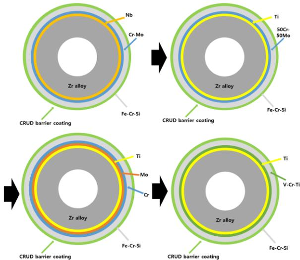
Fig 2. Changes in MMLC fuel cladding design
