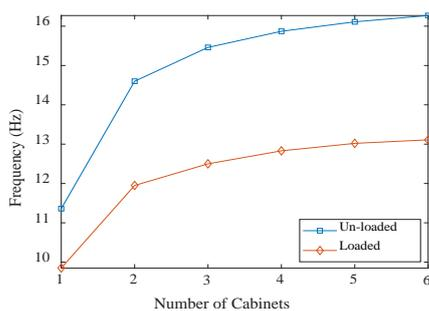
Fig. 2. Effect of the internal components load and number of cabinets.
