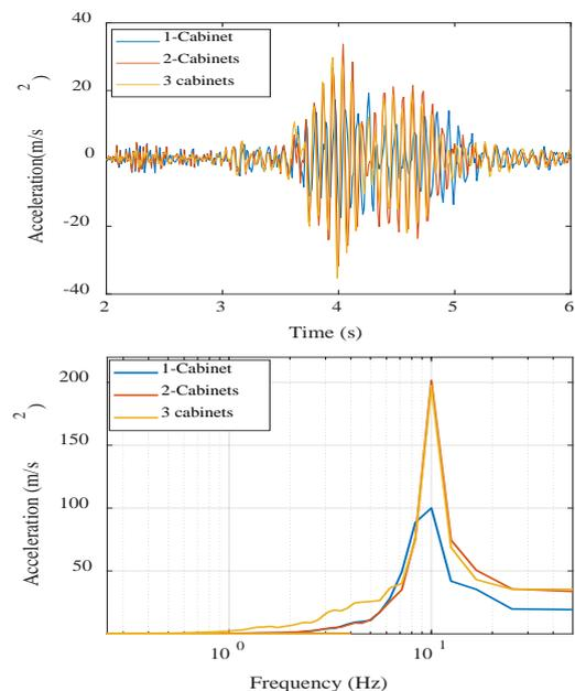
Fig. 4. Cabinet response under the Goungju Earthquake
