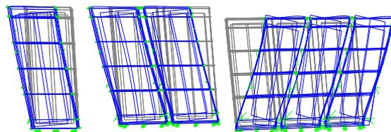
Fig. 1. FE Models of cabinets for the comparative analysis
