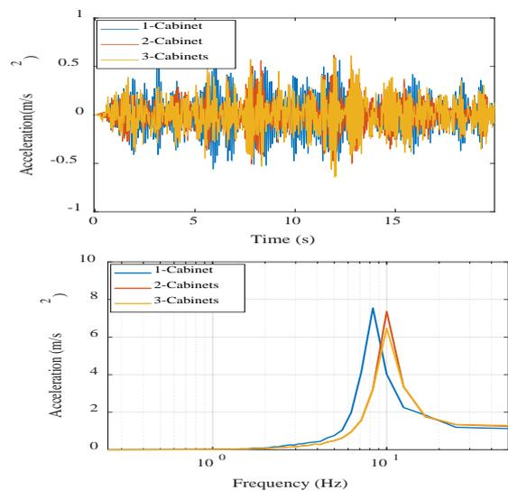
Fig. 3. Cabinet response under the Artificial ground motion compatible with RG 1.60
