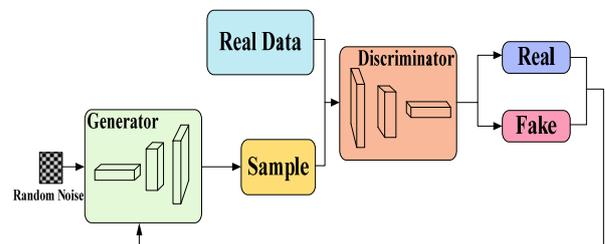
Fig. 1. Overview of the DCGAN Structure
