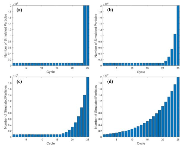
**Figure 1.** Ramp-up modes: (a) step, (b) step-exponential (4 steps), (c) step-exponential (8 steps), and (d) full exponential.
