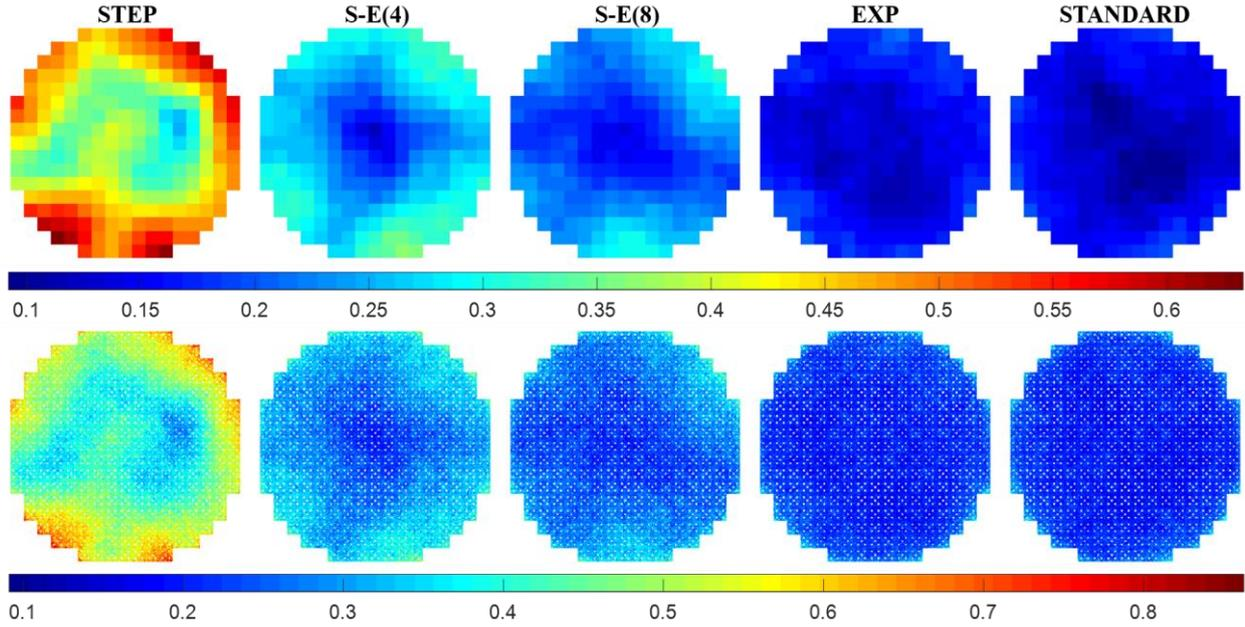
Figure 4. Assembly and pin power real standard deviation (%) distributions.
