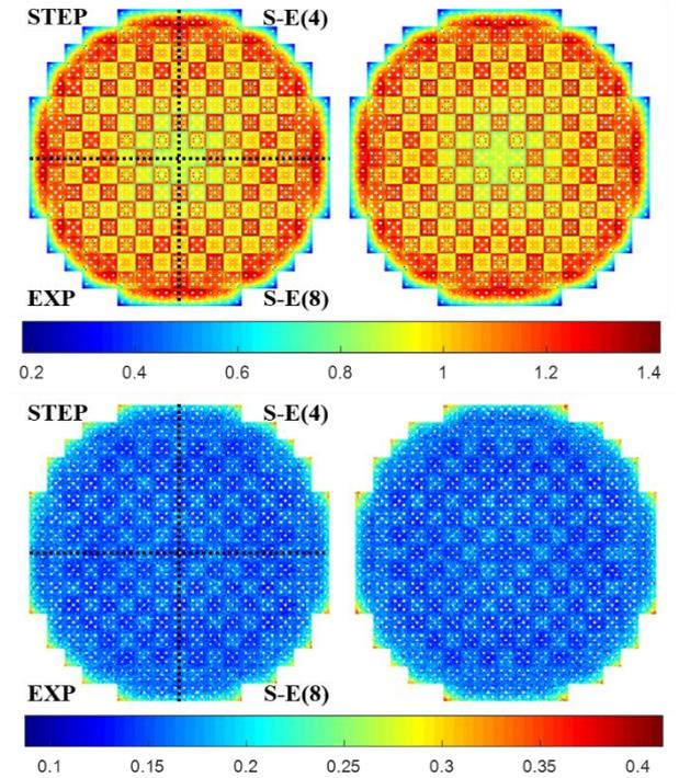
**Figure 3.** Pin power and apparent standard deviation (%) distributions.
