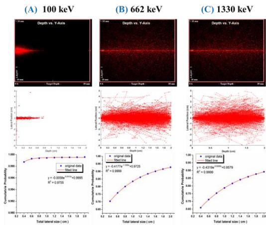
Fig. 3. The stopping and range of ions in matter (SRIM) simulation results for the inspection of scattered photon inside of detector array for different energy of gamma rays (100 keV, 662 keV, and 1,330 keV).
