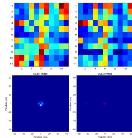
Fig. 6. Detector response map acquired by conventional method (top left) and by new method (top right) testing with Cs-137 located at center and 1 meter source-to-detector distance. And reconstructed images using MLEM for each cases (bottom)
