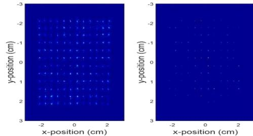
Fig. 4. 2D flood histograms for the 12 x 12 pixels detector array for the Cs-137 located at the center with 1 meter source to detector distance using conventional Anger logic readout (left) and applying new readout method (right).
