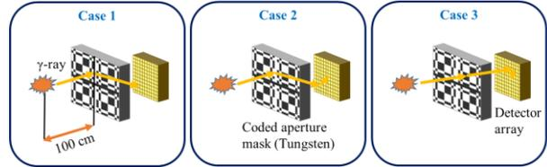
Fig. 1. The cases of Compton scattering events in the coded-aperture imaging system, which increase the probability of blurred reconstructed image and wrong location determination of gamma ray.
