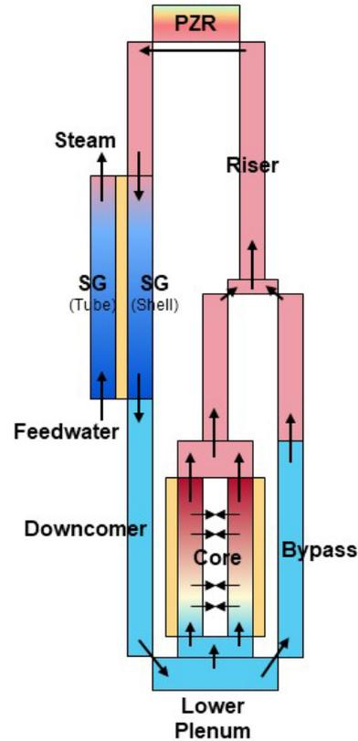
Fig. 1. Nodal structure of the reference SMR
