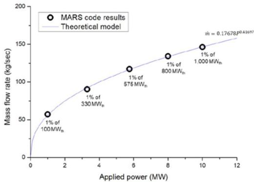
Fig. 2. Mass flowrates with the powers applied to the core
