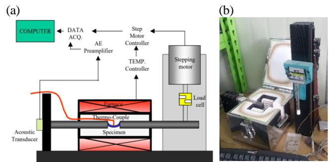
Fig. 2. Schematic illustration of CB tester, (a) integrated computer control system in order to control load and to acquire cracking through acoustic emission (AE) and loading, and (b) photograph of CB testing system.
