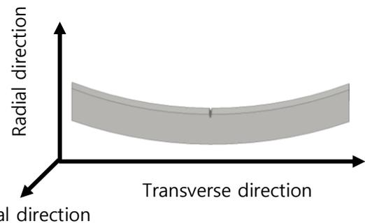
Fig. 1. Geometry of CB specimen machined from Zr-2.5Nb pressure tube.
