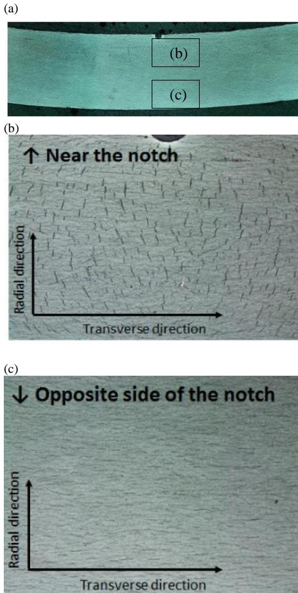
Fig.3. Hydride distribution after reorientation experiment at 350°C under 25 MPa√m.
