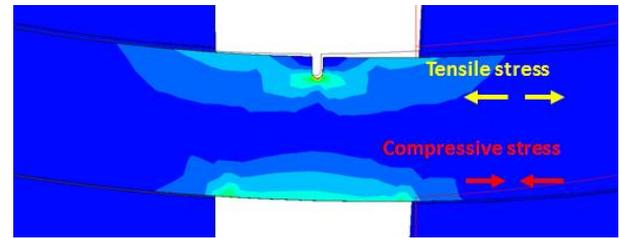
Fig. 4. The schematic illustration of applied stress in CB specimen during reorientation experiment.
