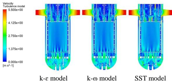
Fig. 5. The velocity distributions of inlet section
