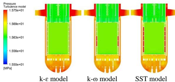
Fig. 3. The pressure distributions of inlet section
