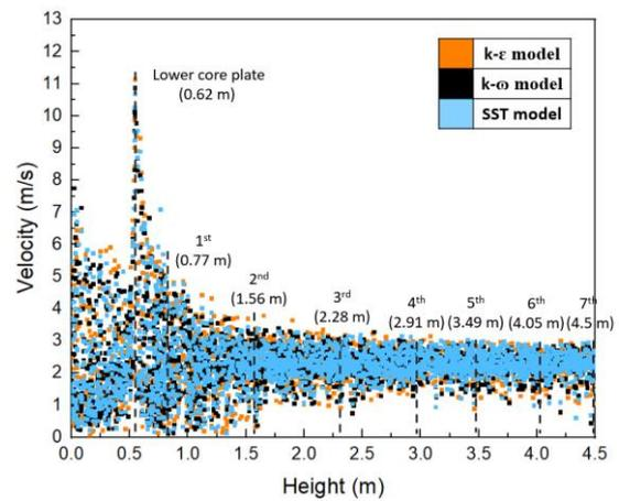
Fig. 7. Velocity profiles of the core region with different turbulence models.
