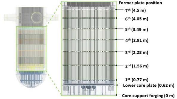
Fig. 2. Positions of baffle structure
