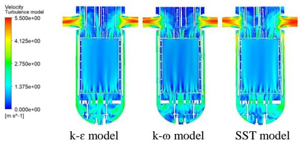
Fig. 6. The velocity distributions of outlet section
