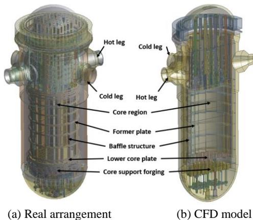
Fig. 1. Schematics of Westinghouse 2-loop reactor
