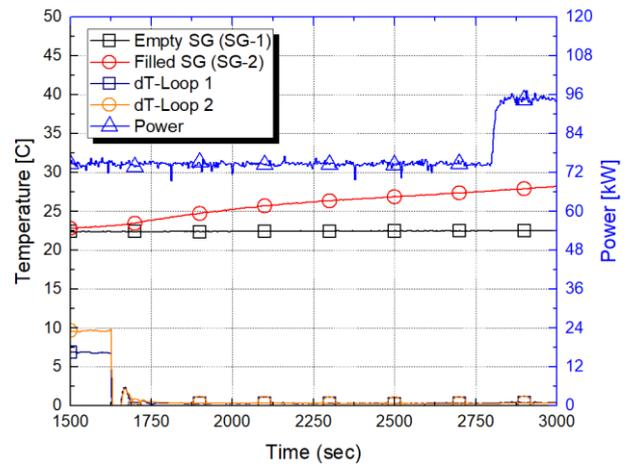
Fig. 3. Variations of temperature differences between hot legs and cold legs, and SGs of the loops with empty and filled SGs under forced convection phase.
