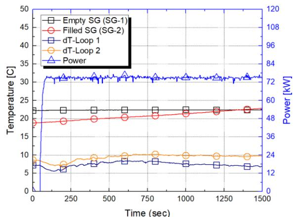
Fig. 2. Variations of temperature differences between hot legs and cold legs, and SGs of the loops with empty and filled SGs under natural circulation phase.
