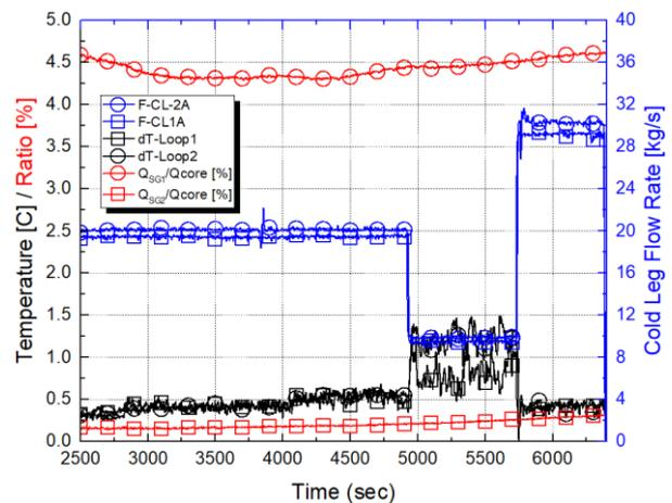
Fig. 4. Variations of temperature differences between hot legs and cold legs, and SGs of the loops and SG's heat removal rates.
