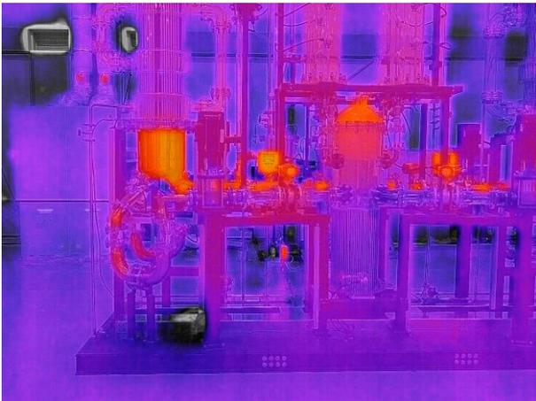
Fig. 5. Temperature field exhibiting different temperature between cold leg and hot leg of URI-LO.
