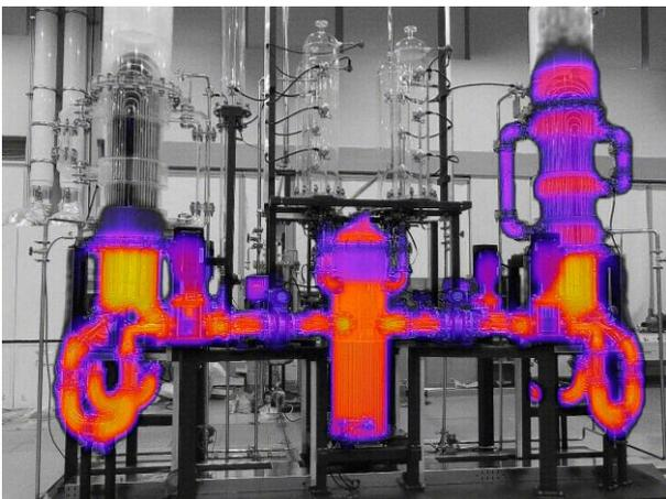
Fig. 6. Overall temperature field of URI-LO during forced convection condition.
