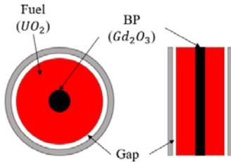
Fig. 2. Cross-section of nuclear fuel containing gadolinium in the form of a cylinder.
