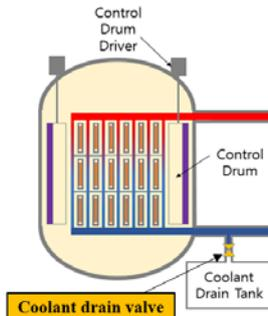
Fig. 3. The coolant drains system of a micro modular water-cooled reactor with a solid core
