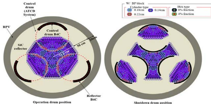
Fig. 1. Cross-section of micro modular water-cooled reactor with a solid core
