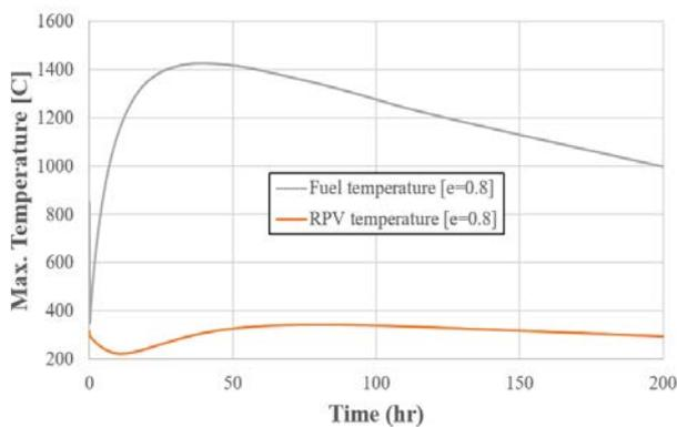
Fig. 7. Nuclear fuel(left) and RPV (right) temperature in a LOCA
