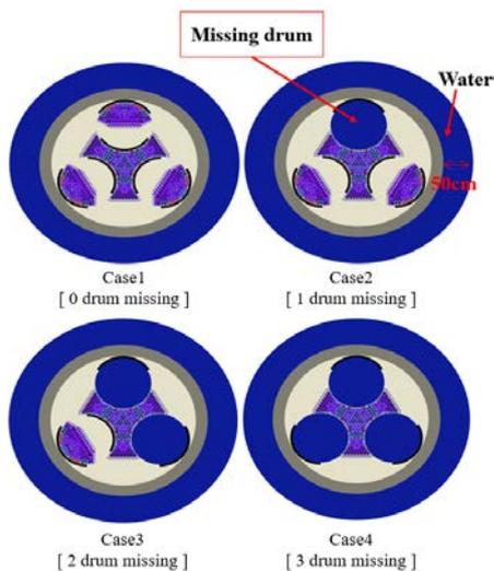
Fig. 5. Reactor flooding scenario during transportation.
