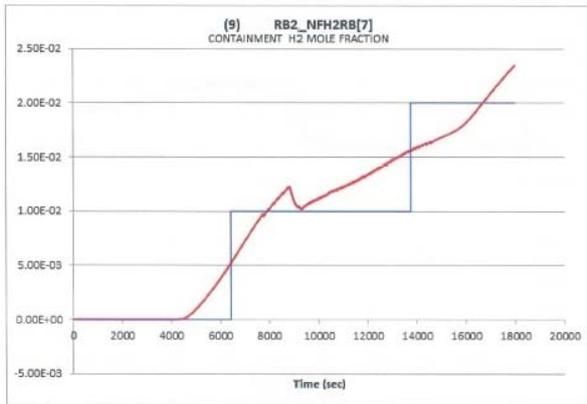
Fig. 1. Containment H2 Mole Fraction, where response of simulator gives continuous trend while stand-alone result shows step-change trend
