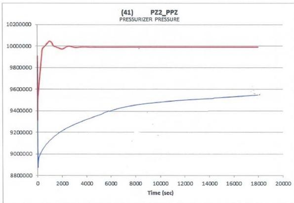
Fig2. Pressurizer Pressure, where stand-alone response is lower than that of simulator due to the lack of heater modeling
