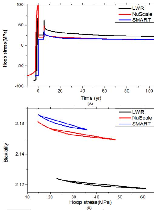
Fig 7. Cladding (A) hoop stress, (B)biaxiality
