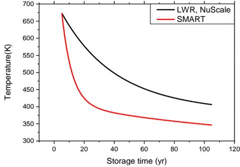
Fig 3. Cladding temperature during dry storage
