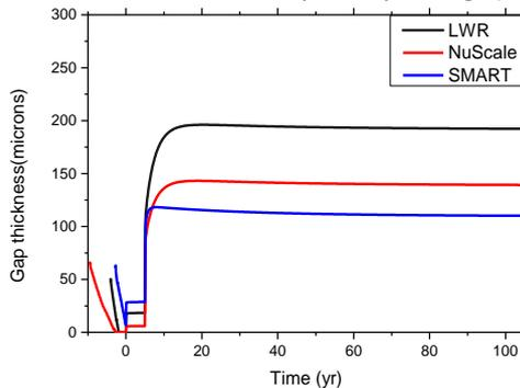
Fig 5. Fuel and cladding mechanical gap thickness
