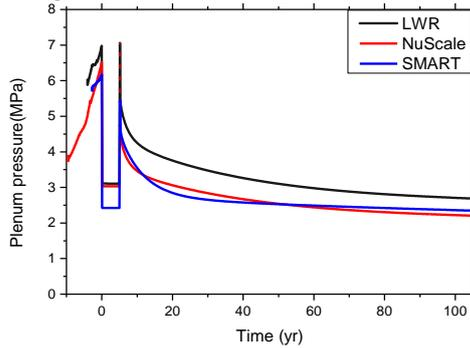
Fig 4. Fuel rod plenum pressure
