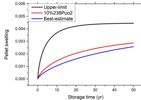
Fig 1. Pellet swelling ( $\Delta a/a_0$ ) after discharge at 60Mwd/kgU [3]
