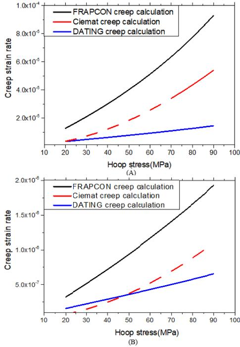
Fig 2. Cladding creep strain rate at (A)400°C, (B)300°C [5]
