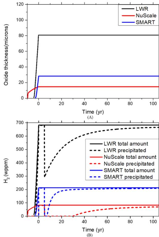
Fig 6. Cladding (A)oxide thickness and (B)hydrogen-pickup and precipitation
