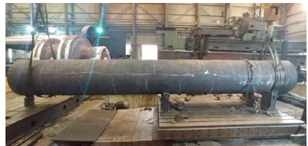
Figure 2. Image of developed SA508 Gr.1A MSL piping
