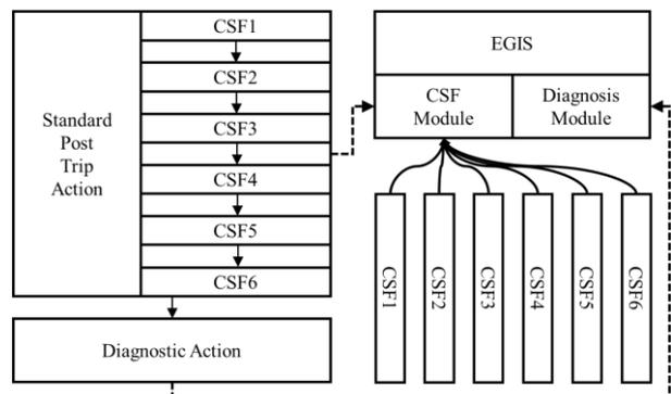
Fig. 2. Comparison between emergency operating procedures and EGIS
