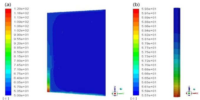
Fig. 5. Temperature[°C] distribution of the plane(a) and the MSPT(b)
