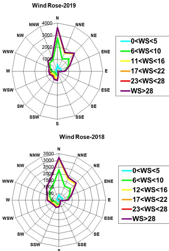
Fig. 2. Wind rose diagram in 2019 and 2018
