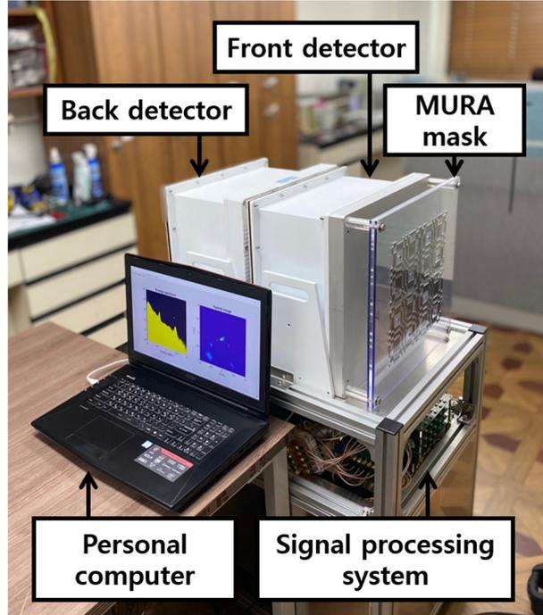
Fig. 1. Developed LAHGIS composed of two NaI(Tl) scintillation detectors, a MURA mask, a signal processing system and a personal computer.
