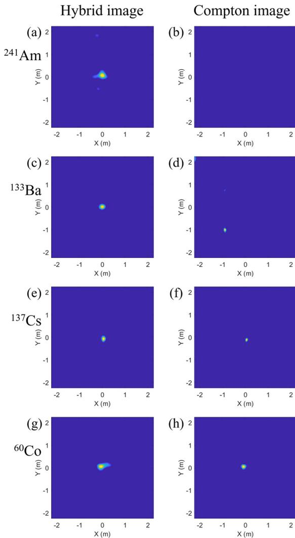
Fig. 2. Reconstructed images of the sources with different gamma energies: (a, b) 59.5 keV of  $^{241}\text{Am}$ , (c, d) 356 keV of  $^{133}\text{Ba}$ , (e, f) 662 keV of  $^{137}\text{Cs}$ , and (g, h) 1170 and 1330 keV of  $^{60}\text{Co}$ ; hybrid images (left) and Compton images (right).
