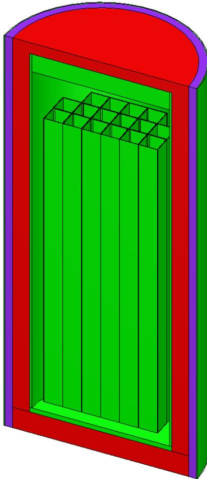
Fig. 1. Geometry Configuration of OASIS-32D cask Model (Front-half Cut)
