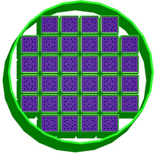
Fig. 2. Geometry Configuration of OASIS-32K Canister Calculation Model (Top-half Cut)
