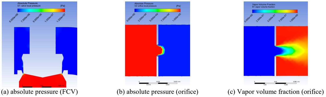
Fig. 3 CFD results - case 3: reference case
