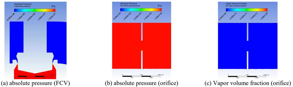
Fig. 4 CFD results - case 1: case of stable flow rate
