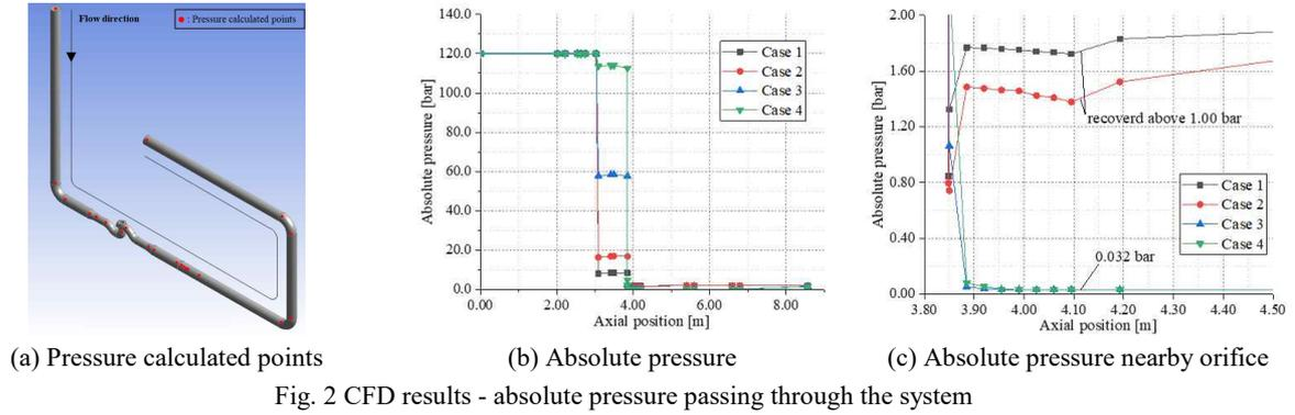
Fig. 2 CFD results - absolute pressure passing through the system
