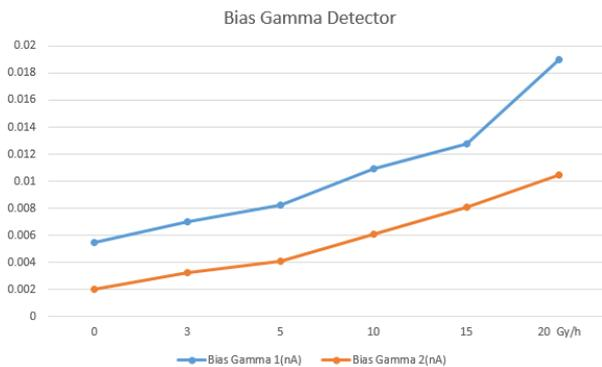
Fig. 5. Current measurement of bias gamma-ray detector.
