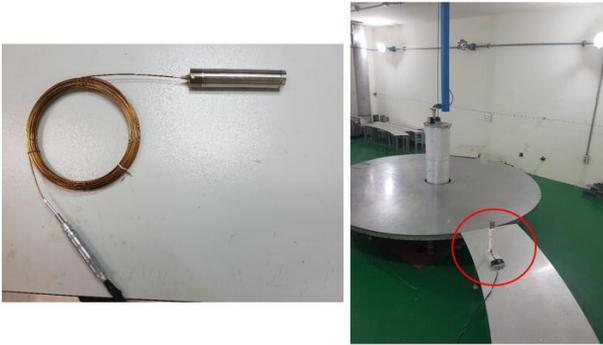
Fig. 3. Bias Gamma-ray Detector (left) and Gamma-ray irradiation test (right)
