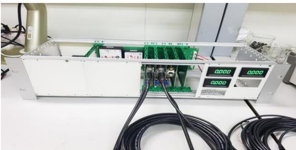
Fig. 4. Picoammeter for nA current measurement
