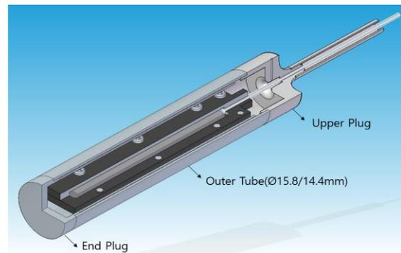
Fig. 1. Design of bias gamma-ray detector
