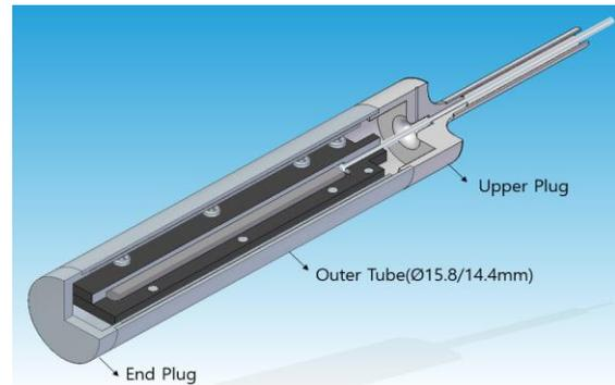
Fig. 1. Design of bias gamma-ray detector
