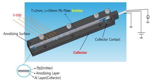
Fig. 2. Current measurement principle of bias gamma-ray detector
