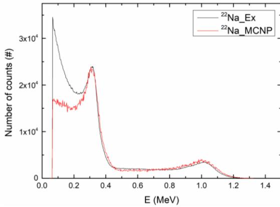
Fig. 1. Measured and simulated energy spectrum with <sup>22</sup>Na
