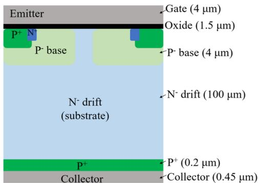
Fig. 1 A schematic vertical structure of the IGBT device.
