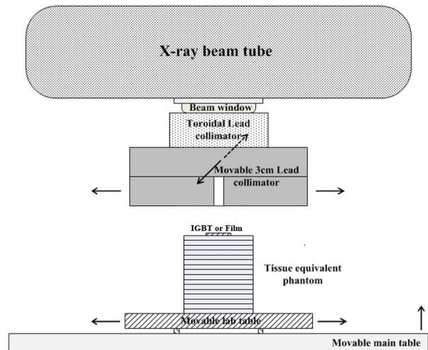
Fig. 2 A schematic of the X-ray irradiation system.
