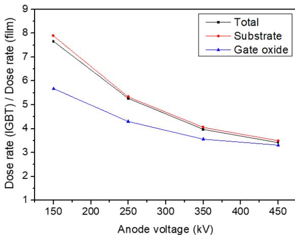
Fig. 3. The ratios of the IGBT inner layers' dose rate to the gafchromic EBT film's dose rate at 150, 250, 350, and 450 kV anode voltage.
