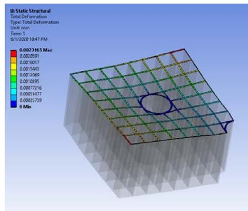
Figure 8 Total deformation case 2
