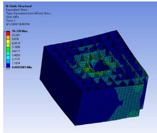
Figure 9 Equivalent stress case 2
