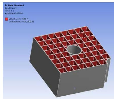
Figure 4 Setting up the force boundary condition
