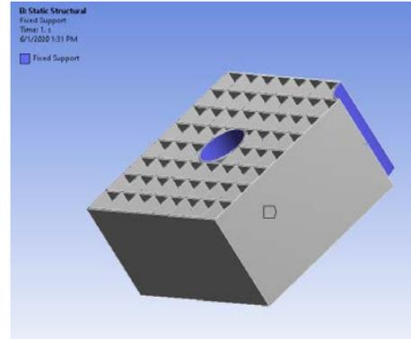
Figure 3 Setting up a fixed support boundary condition
