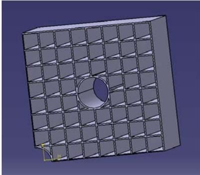
Figure 1 Quarter 3D model of the mid grid
