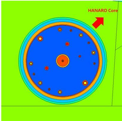
Fig. 2. Selected SPND arrangement (MCNP model)
