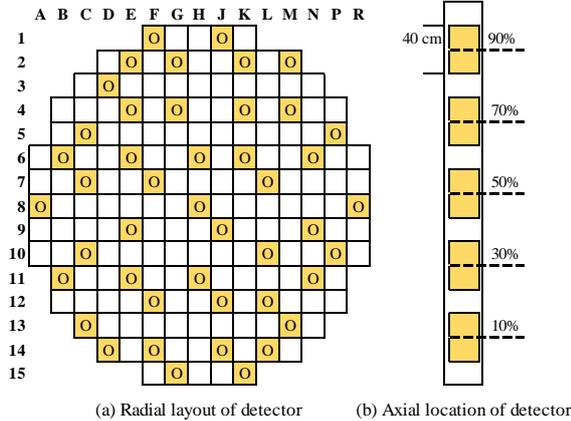
Figure 4 Detector position in OPR-1000
