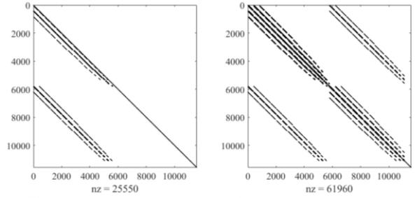
**Figure 1** Non-zero matrix of incomplete Cholesky factorization
