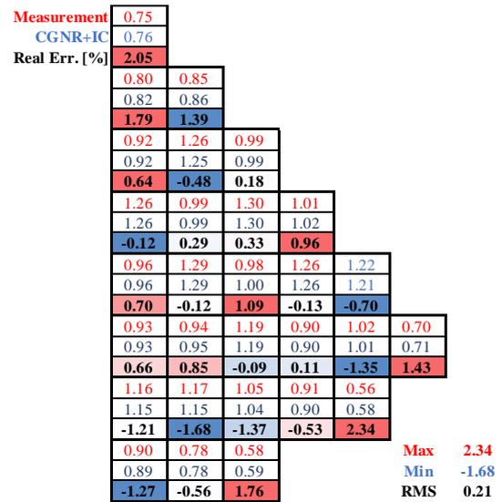
Figure 6 Radial power shape [5 GWd/MTU]
