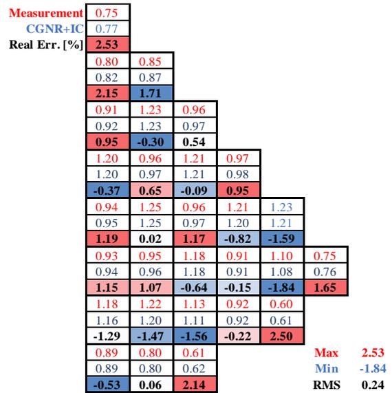
Figure 7 Radial power shape [10 GWd/MTU]
