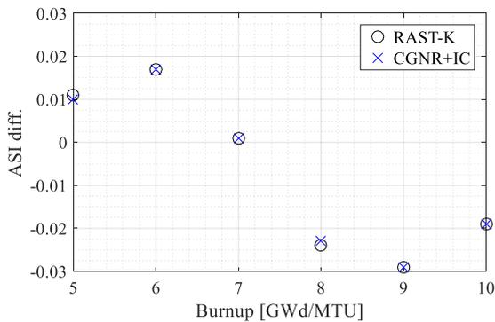
Figure 8 Comparison of Axial Shape Index
