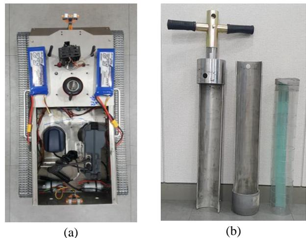
Fig. 1. The Measurement System for detecting concentrations of residual radioactivity (Unmanned Vehicle for Detection(a), Soil Sampling Equipment(b))
