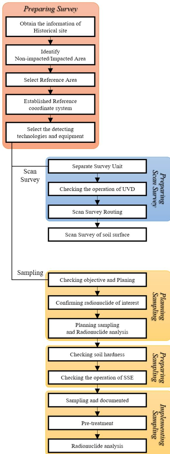
Fig.2. The Survey Procedures for the Detecting Concentrations of Residual Radioactivity
