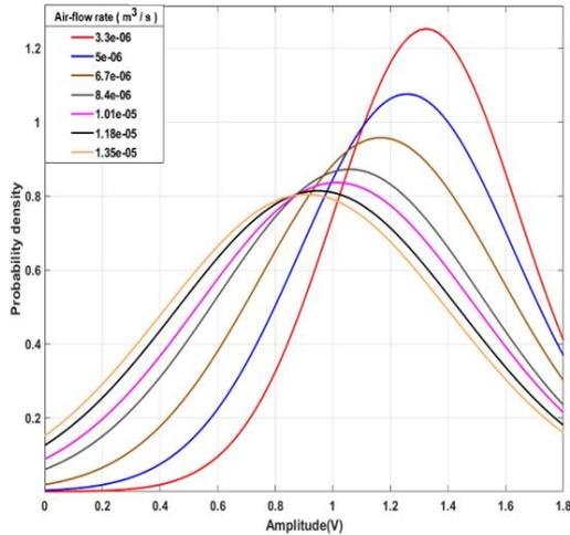
Fig. 3. Probability distribution of A5 amplitude analyzed by 25000 data sets for each air flow rate.
