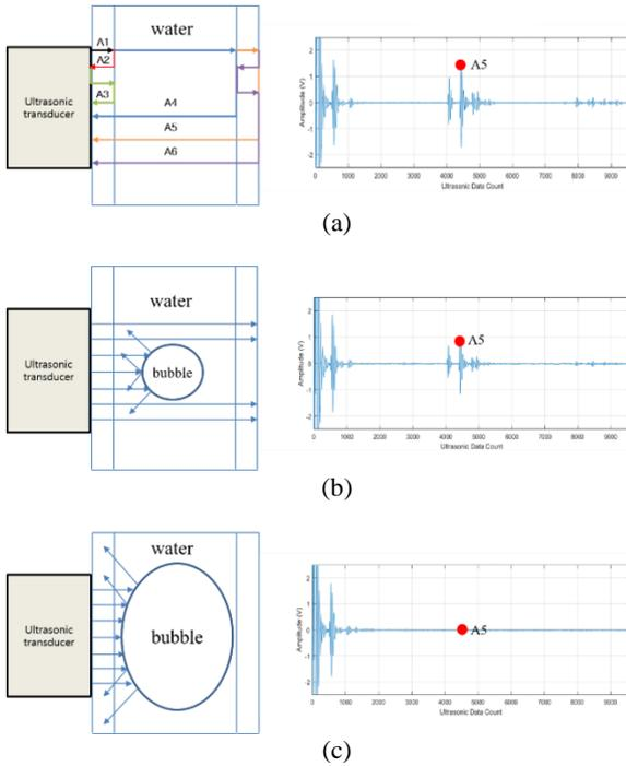
Fig. 2. The ultrasonic signal in the test section (a) only water (reference) (b) small bubble (c) large bubble.
