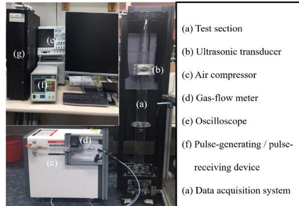
Fig. 1. Experiment apparatus for measuring bubble detection.
