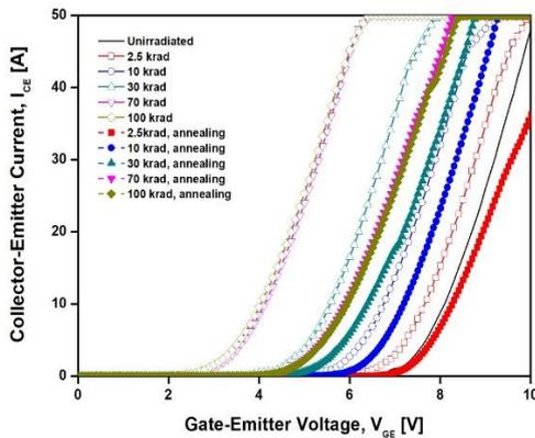
Fig 2. Gate-emitter voltage and collector-emitter current transfer curves for gamma-ray irradiation dose with and annealed.
