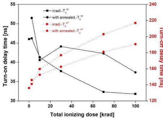
Figure 5 Turn-on and turn-off delay time due to gamma-ray irradiation dose and annealing.
