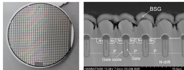
Fig 1. (a) Fabricated 6-inch NPT-trench gate IGBT wafer (b) Cross-section image of NPT-trench gate IGBT obtained using FE-SEM
