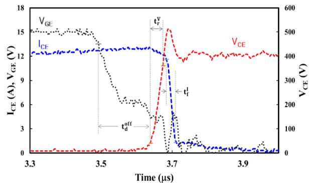
Fig 4. Switching time waveforms of the turn-off (b)  $t_d^{off}$ ,  $t_f^I$ ,  $t_r^V$
