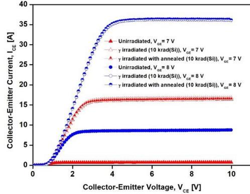
Fig . Collector-emitter voltage and current curves at a gate voltage of 7 and 8 V for the unirradiated and irradiated (10 krad (Si)) and thermal annealing device
