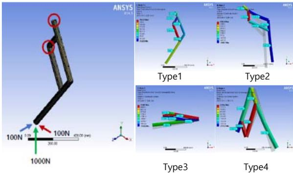
Fig. 3. A static FEM analysis model and results for 4 support conditions.
