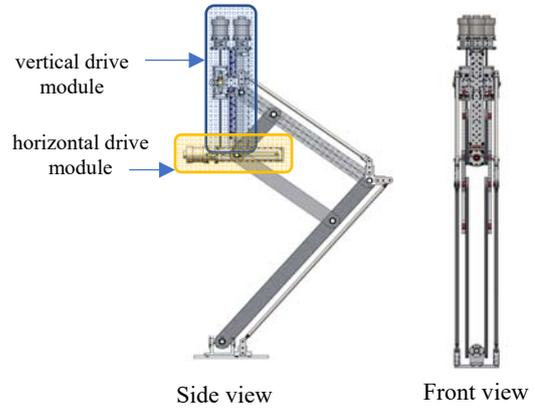
Fig. 4. The proposed pantograph leg design.
