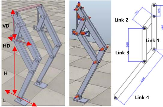
Fig. 2. 2DOFs pantograph leg mechanism.
