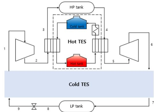
Figure 2. Schematic of CCES
