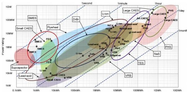
Figure 1. Comparison of power rating and rated energy capacity with discharge time duration at power rating [2]
