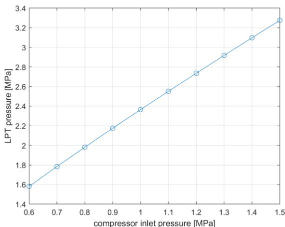
Fig. 5. Effect of compressor inlet pressure on LPT pressure
