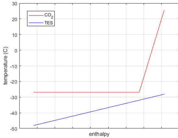
Figure 3. Temperature profile in cold TES when compressor inlet pressure is 0.6 MPa
