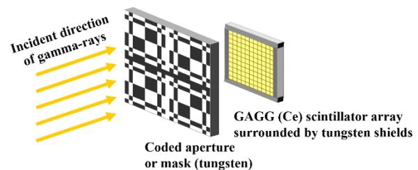
Fig. 2. Simulation geometry used in the Monte Carlo calculation for the gamma-ray response of EPSILON-G.
