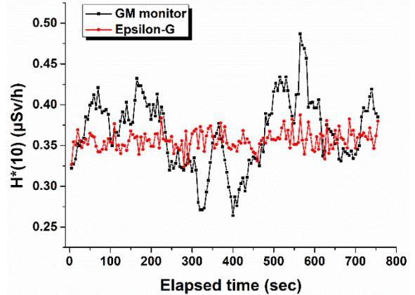
Fig. 4. Comparison of the ambient dose equivalent rate,  $H^*(10)$ , over time obtained with EPSILON-G (red) and a GM monitor (black).
