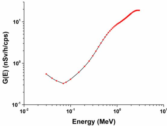
Fig. 3. The factor for converting the measured pulse height spectrum to ambient dose equivalent calculated using  $50 \times 50$  response matrix.
