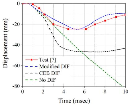
Fig. 2. Comparison of displacement-time histories between test and analysis results
