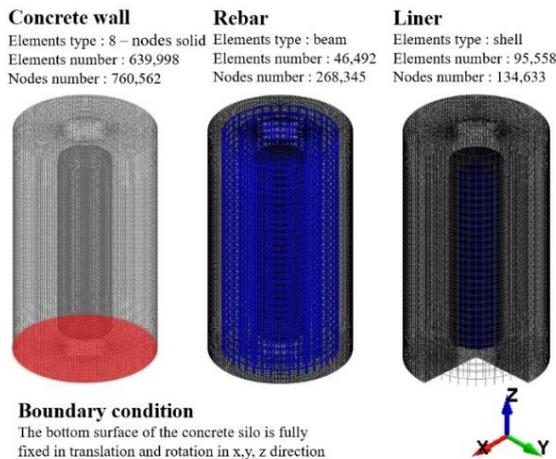
Fig. 3. FE models of concrete silo
