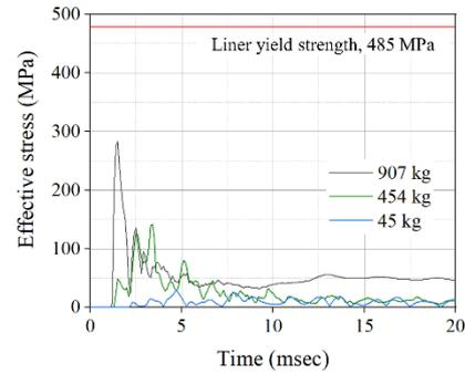
Fig. 4. Comparison of effective stress histories of liner for each charge weight
