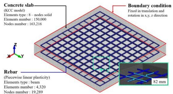
Fig. 1. Schematic of RC specimen [7]
