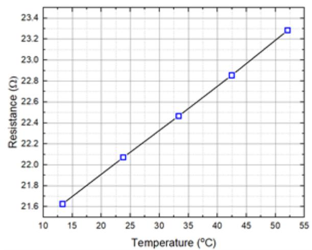
Fig. 4. RTD calibration results of 50 nm thick Pt heater on fabricated AAO membrane.
