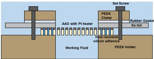
Fig. 2. Schematics of R123 pool boiling experiment test section with AAO membrane based nano porous heater.
