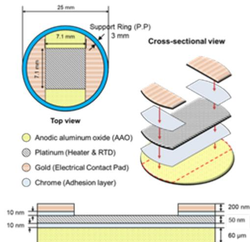
Fig. 1. Schematics of AAO membrane based nano porous heater assembly in current study.
