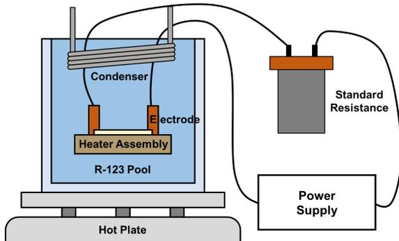
Fig. 3. Schematics of R-123 pool boiling experimental apparatus setup.
