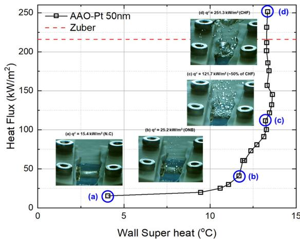
Fig. 5. R123 pool boiling curve of Pt deposited AAO membrane based nano porous heater assembly.
