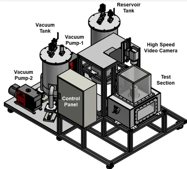
Fig. 6. Thin film boiling experimental facility.
