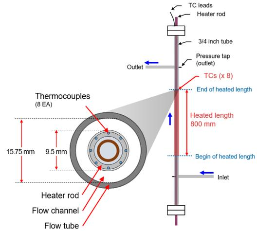
Fig. 3. Configuration of test section
