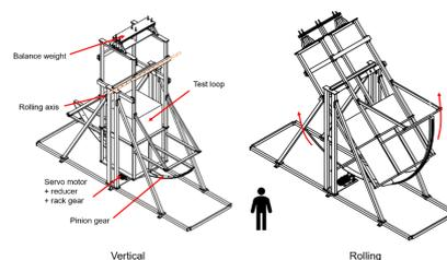
Fig. 1. Configuration of rolling platform, NEOUL-R
