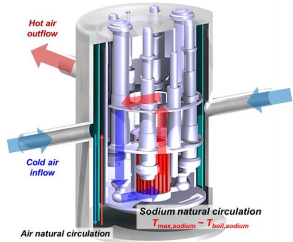
Fig. 1. Schematic of the RVACS in the PGSFR [5]
