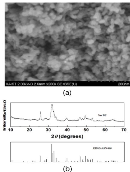
Figure 1. (a) SEM image of synthetic HAP nano-particles (b) XRD pattern of synthetic HAP.
