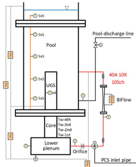
Figure 2. Schematic of the experimental apparatus
