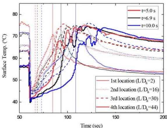
Figure 4. Heater surface temperatures in the edge sub-channel
