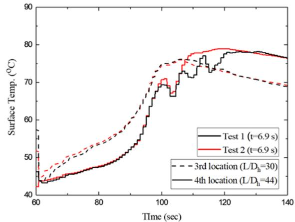
Figure 5. Comparison of heater surface temperature between repeatable tests
