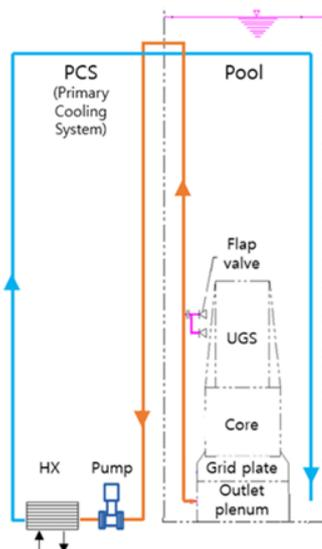
Figure 1. Schematic of PCS of the research reactor
